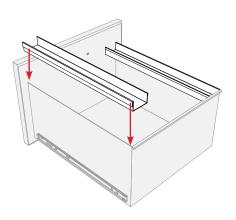
Wider drawers have single center adapter. Remove the appropriate existing screws, then reinstall them holding the adapter in place.
