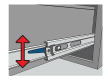
Narrower drawers will have two adapters that slide over the edges of the drawer sides
