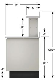
\* HEIGHT SHOWN IS BASED ON A 1 1/4" THICK WORK SURFAC OVERALL HEIGHT VARIES DEPENDING ON THICKNESS
