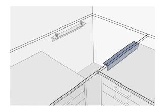
Countertop Support Brackets - Adjustable Height for mounting onto wall:
