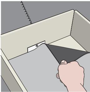
An integral component of a Teclab ESD work station is the **Grounded Cabinet**. Each drawer has a coiled Ground Wire connected to a Ground Bracket installed on the cabinet shell to dissipate static. The cabinet is then connected to the Common Point Ground System.
