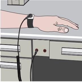
Human handling is responsible for approximately 90% of all ESD damage, so use of a **ESD Wrist Strap** is essential. The ESD Wrist Strap features a conductive thread interwoven on the breathable elastic band that provides 360° of skin contact.
