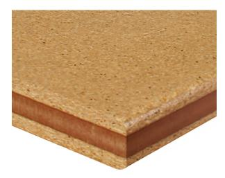
**RESINWOOD WORKSURFACES AND SHELVES** shall be 1 %" thick. Work surfaces and shelves are available in sizes up to 60" x 144". Work surfaces and shelves shall be installed with a uniform 1" (25mm) overhang on the front and exposed ends. All front edges shall be finished with a %" radius edge. A 180° bullnose front edge is also available.
